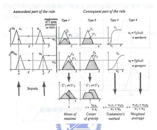
Figure 2-3 Diagrammatic representations of defuzzification methods (Passino and Yurkovich, 1997).
