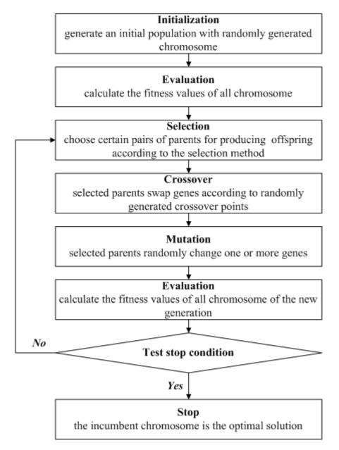
Figure 2-4 Typical operation of a GA.
