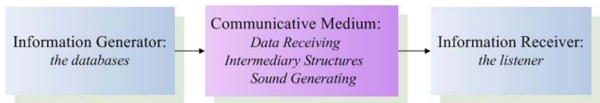
Fig. 5 Schematic of an Auditory Display System
