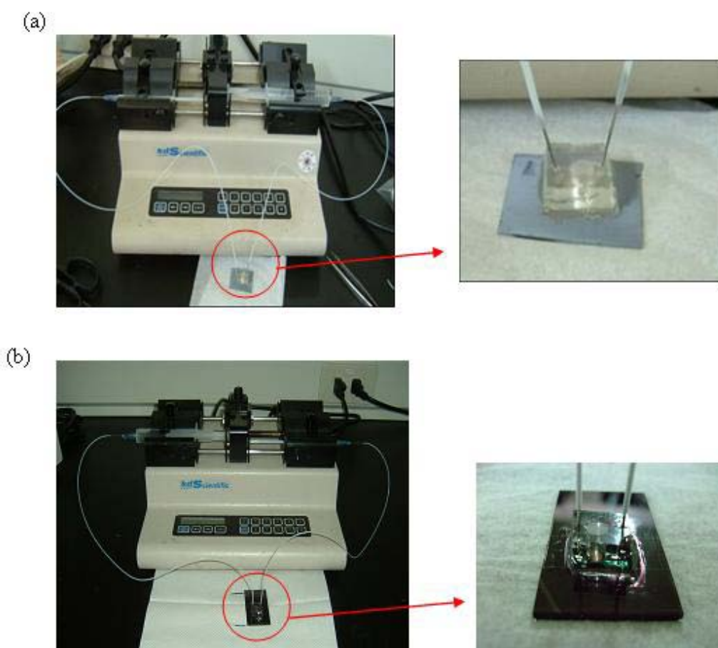
Figure 3-20 Schematic of the testing apparatus used for microfluidic system with syringe pump. (a) is microfluidic reactor with textured surface by TMAH, and (b) is textured surface of solar cell.
