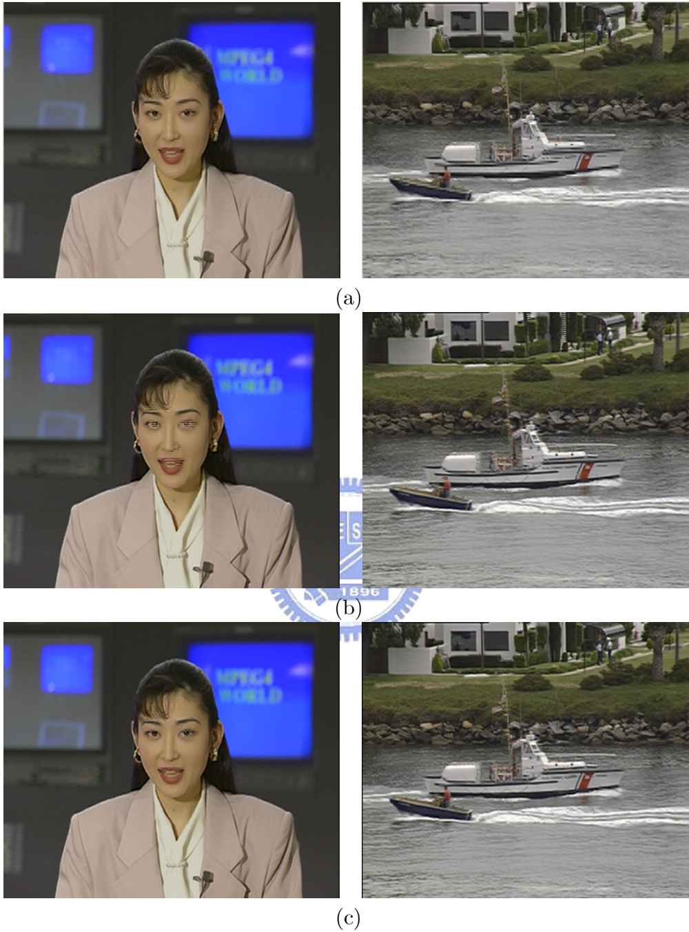
Figure 4.7: The experiment result for sequence "Aikyo", "Coastgurad."(a) Isophote interpolation. (b) Motion Compensation. (c) Hybrid.
