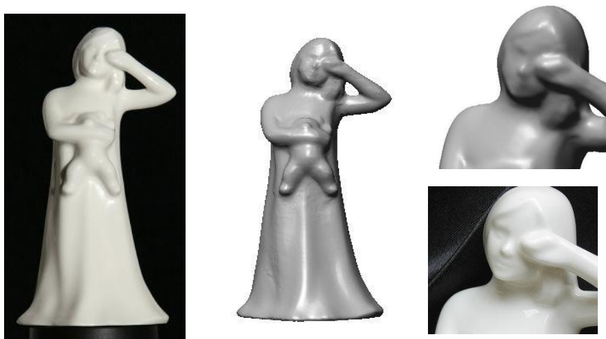
Fig9. Detailed surface reconstructed by Carlos et al's photometric
