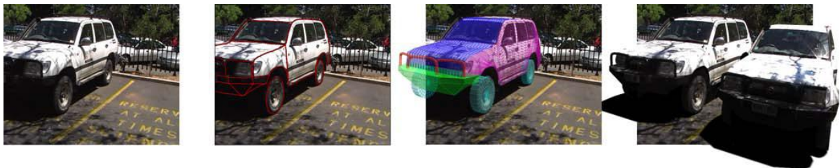
Fig1. Left to right: a frame from the input video sequence, a partial tracing of the model, the final model overlaid on the video, and the result of rendering the final model back into the original sequence.
