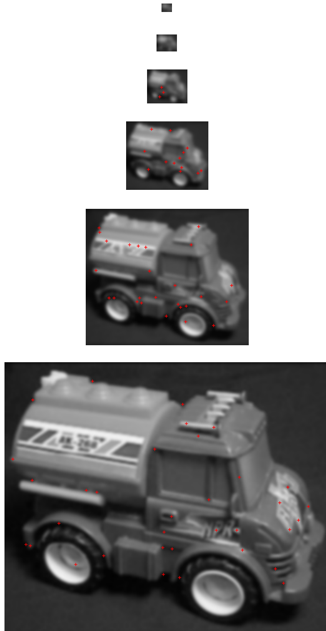
Figure 4.2: SIFT feature points of truck image in Gaussian spaces. SIFT feature points found in different scale level of Gaussian space are marked as crosses.
