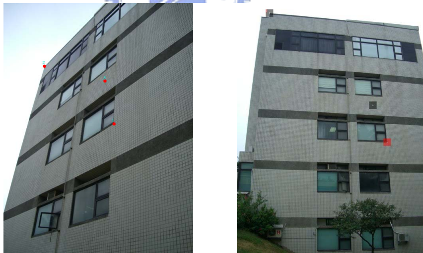
Figure 4.13: Range of point refinement in building images using spiral descriptor. Red points on the left image and the white circles on the right image are the correspondences selected manually. The red/black regions are the points can/can't be refined to the corresponding white circle in a 19 \times 19 searching range within 1.5 pixels error.
