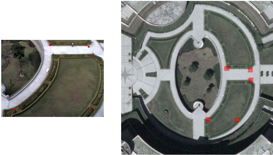
Figure 4.10: Range of point refinement in grassland images using spiral descriptor. Red points on the left image and the white circles on the right image are the correspondences selected manually. The red regions are the points can be refined to the corresponding white circle in a 19 \times 19 searching range within 1.5 pixels error.
