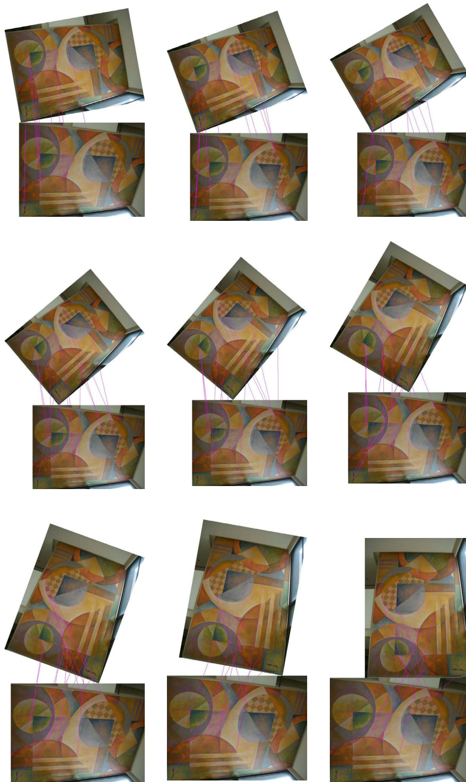
Figure 4.8: Rotation testing for SIFT in wall images. Two wall images are matched using SIFT from 10^\circ to 90^\circ .
