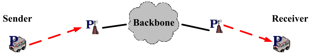
Figure 4.1: A SMFS scenerio in which the source node can directly communicate with a RSU node
