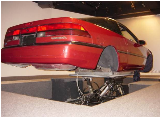
Figure 2-1: The dynamic VR driving environment. (A): the photograph shows the 3D surrounded VR scene. (B): the photograph shows the Stewart platform. (C): the photograph shows locations of the buttons for subjects to select the homing direction and angle.
