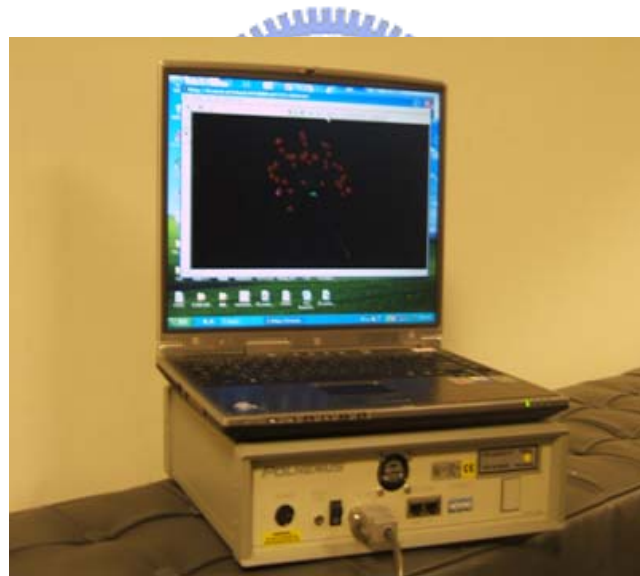
Figure 2-4: The picture shows the 3D Digitizer system which is for digitizing the positions of electrodes. The positions of each electrode are shown as red points on the screen.
