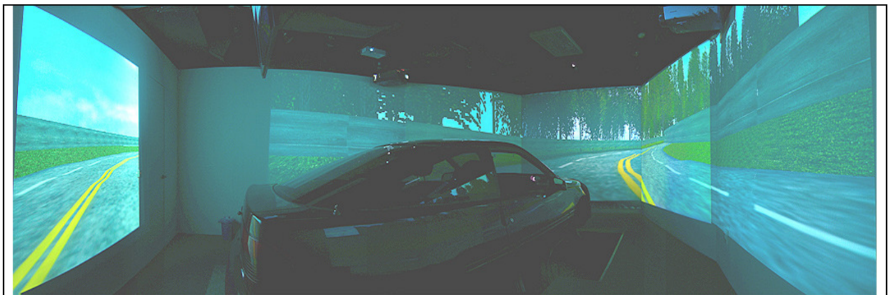
Figure 2-1: The overview of the dynamic VR environment, Brain Research Center, National Chiao-Tung University, Taiwan, ROC. The dynamic VR environment consists of three elements: (1) a six-degree-of-freedom Stewart motion platform; (2) a real car; and (3) a 360-degree 3D VR scene consisting seven projectors. The movements of the platform are according to the car dynamics and the condition of the road surface.
