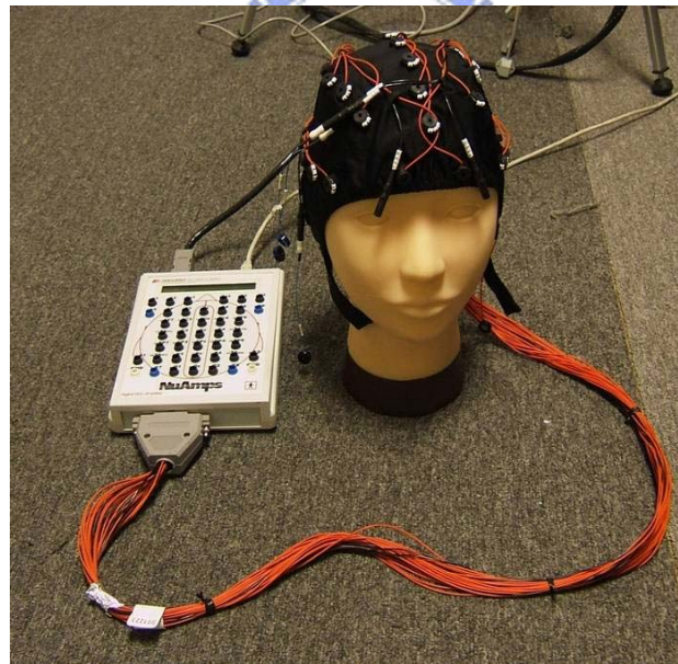
Figure 2-6: The electrode cap and the EEG signal amplifier.
