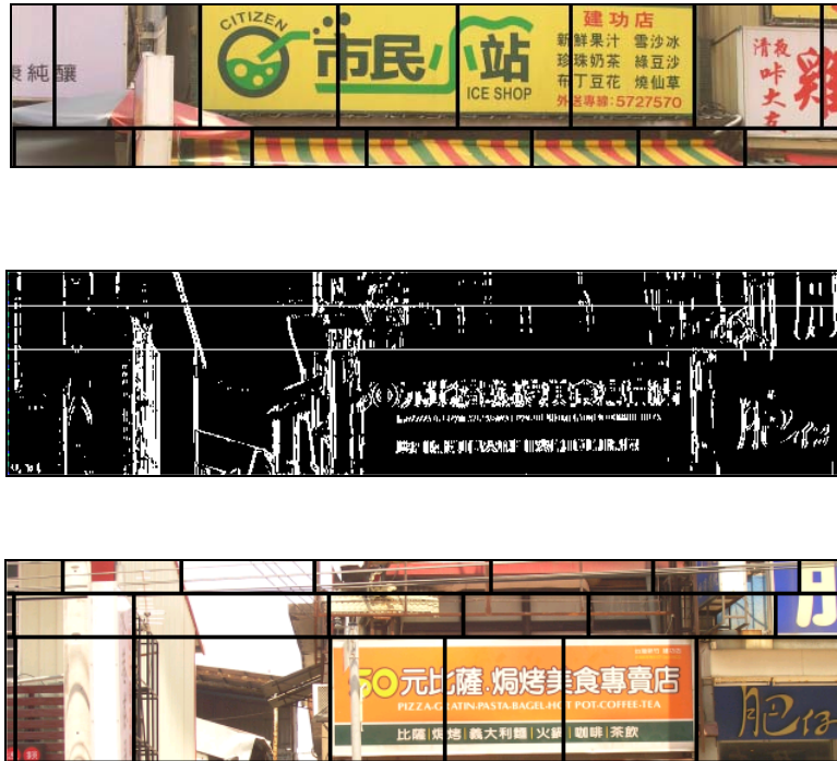
Figure 2-11 Sobel vertical edges maps and first vertical edges selection
