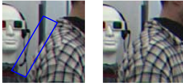
Figure 3-9: The occluded area in the left image can not be seen in the right image.
