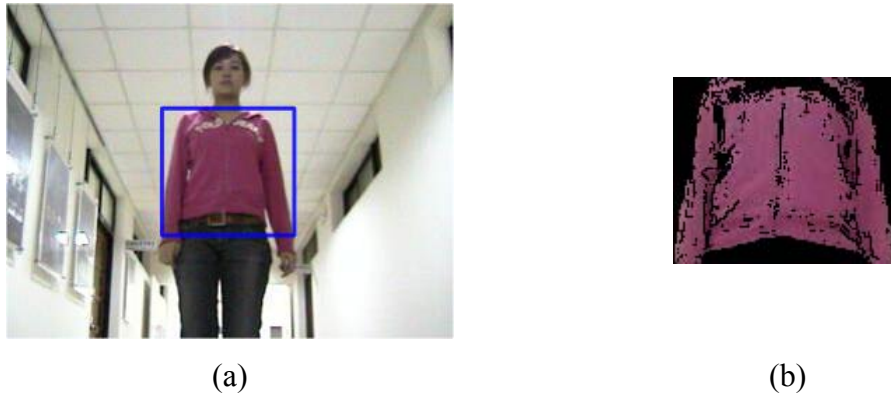
Figure 7.2 An experimental result of extraction of the clothes. (a) The input image. (b) The image of the extracted clothes.
