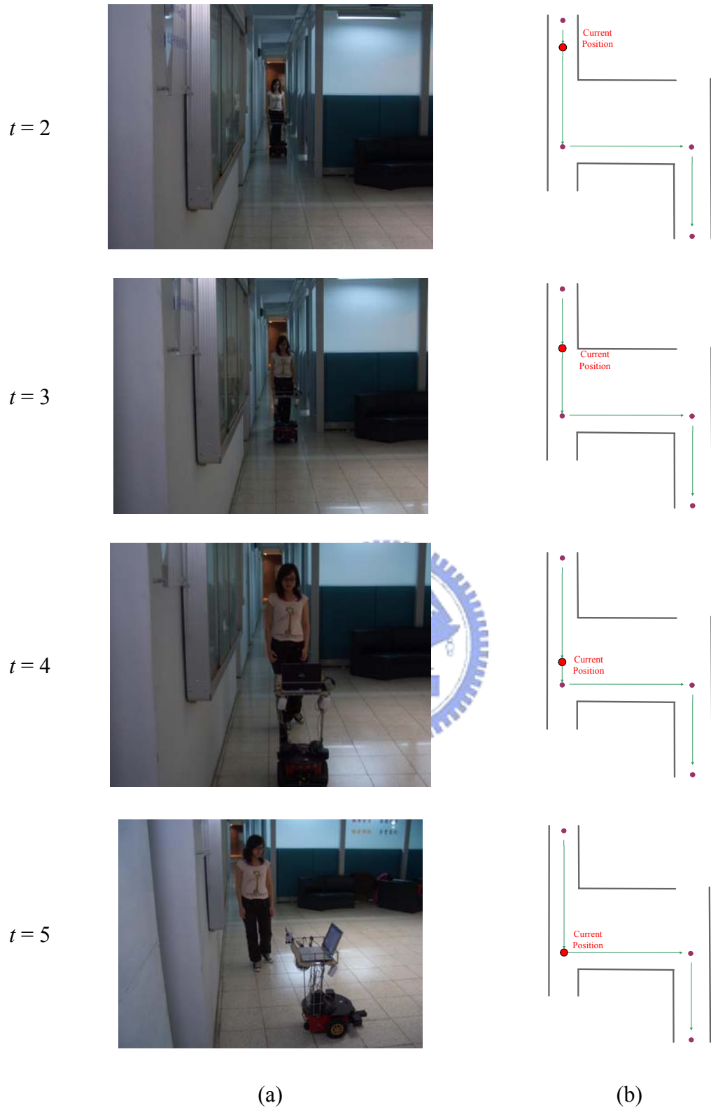
Figure 6.7 An experimental result of navigation in an indoor environment. (a) The vehicle navigates on the path. (b) The navigation map. (continued)
