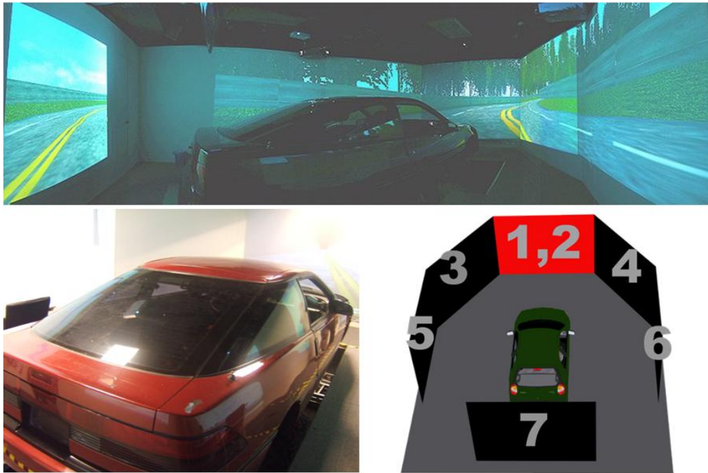
Figure 1. The overview of surrounded VR scene. The VR-based highway scenes are projected into surround screen with seven projectors.
