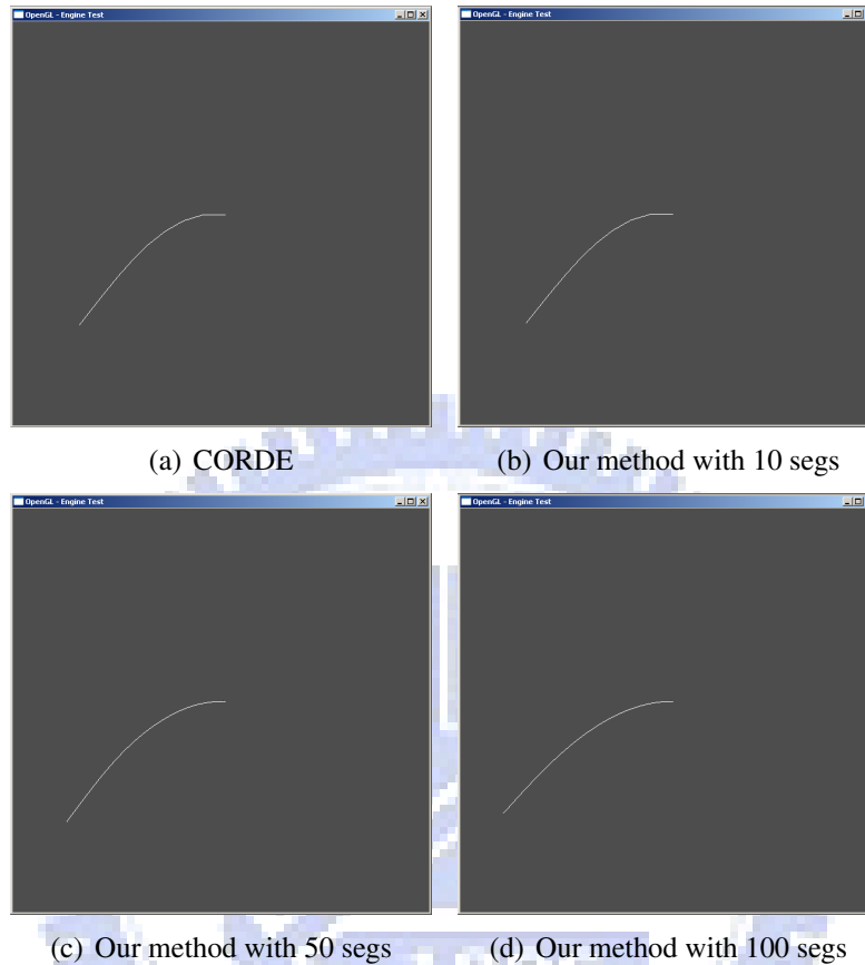
Figure 5.1: Statics Test: Young's modulus is set as 10MPa, and shear modulus is 5MPa. The error of our force transport may increase as the segment numbers increases.
