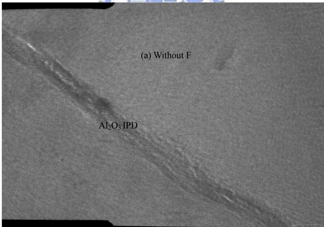
Fig. 2.19 The TEM cross-sectional images of Al 2 O 3 inter-poly capacitors about 100Å ~120Å. (a) without fluorine. (b) FG with 5E13 cm -2 (c) CG with 5E15 cm -2 .
