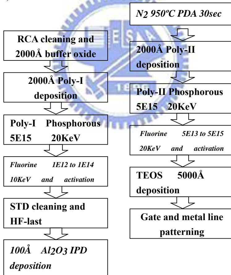
Fig. 2.2 Key process steps of Al 2 O 3 inter-poly capacitors with surface fluorine passivation.
