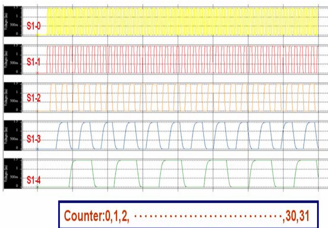
Fig. 3.28 Simulation result of the five bits counter.
