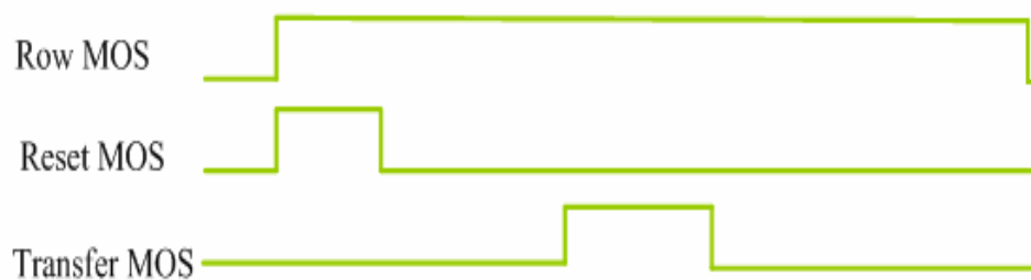
Fig. 3.6 The clock flow of 4-T APS.
