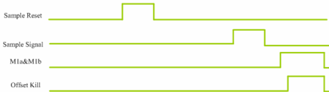
Fig. 3.15 The clock flow of CDS circuit.
