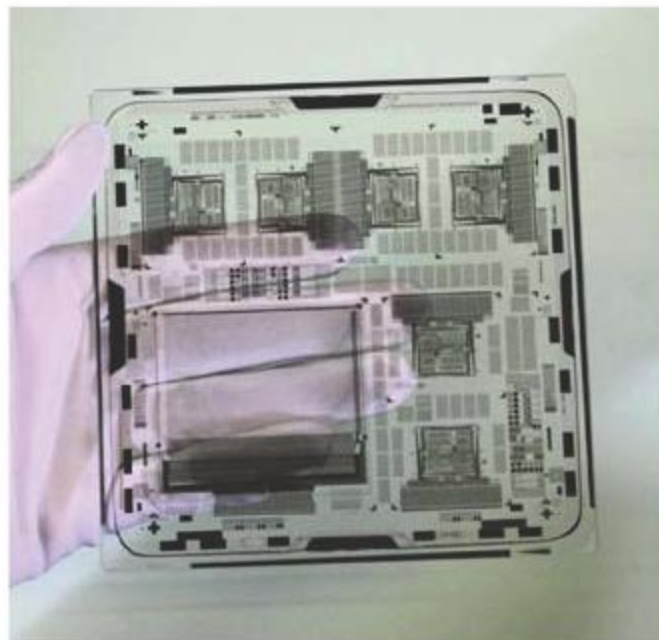
Fig. 1.2 A CPU with an instruction set of 1-4bity and 8-bit data bus on glass substrate [2].
