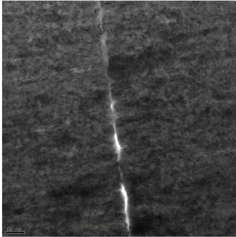
Fig 4-21 TEM image of bonding interface with voids
