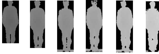
Fig-4.6 Comparison of the result of normalization. The human is originally standing at 1.6m, 2.0m, 2.4m, 2.8m, 3.2m and 3.6m from left to right.
