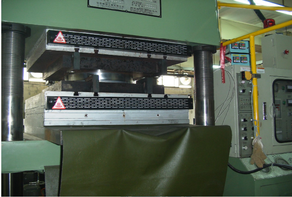
Fig.3-1. The picture of the 40 tons press equipment and the 400mm diameter mold.
