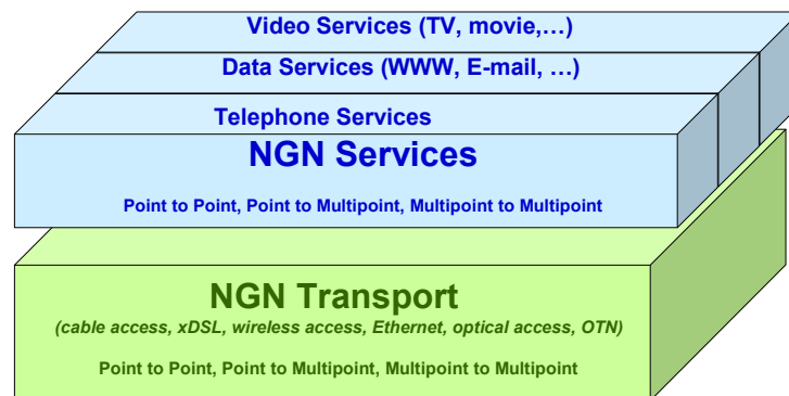
Figure 2 - ITU-T Y.2011 – Separation of services from transport in NGN
