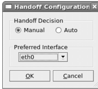
Figure 5.5: The handoff configuration interface.
