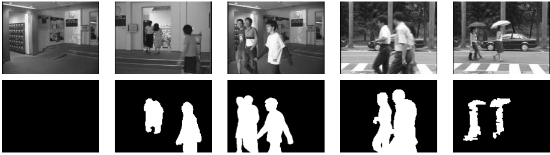
Figure 2.4: Training images for background model initialization. Examples of collected images and their binary maps of the foreground (white) and the background regions (black) are plotted, top and bottom, respectively.
