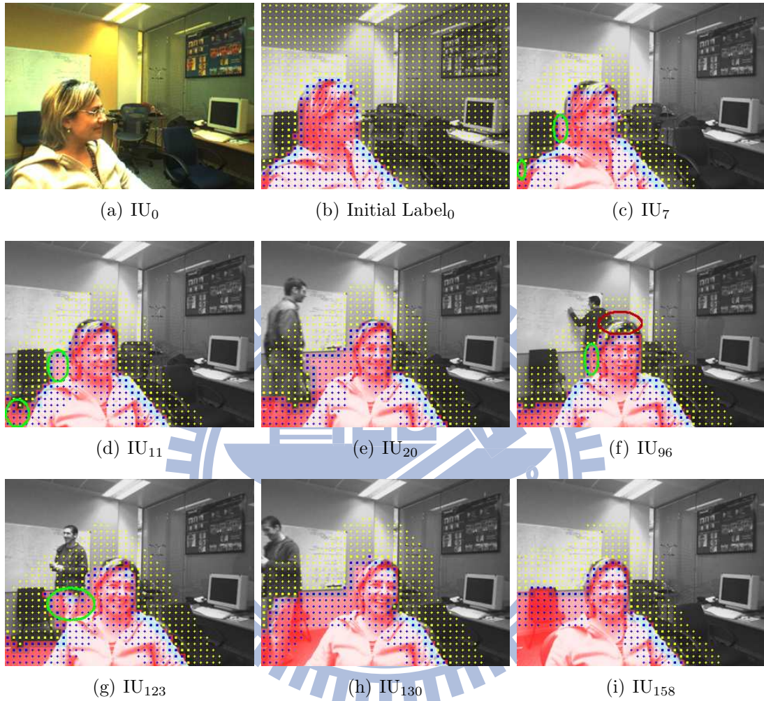
Figure 4.6: Results of the IU experiment. (a) The first image frame of the IU sequence. (b) The initial layer label mask. (c)-(i) Snapshots of the video layer propagation results for the IU sequence. While the brown circle marks the propagation errors due to undifferentiated regions (similar color distributions between the hair and the wall), the green ones indicate the errors resulting from uncovered regions.
