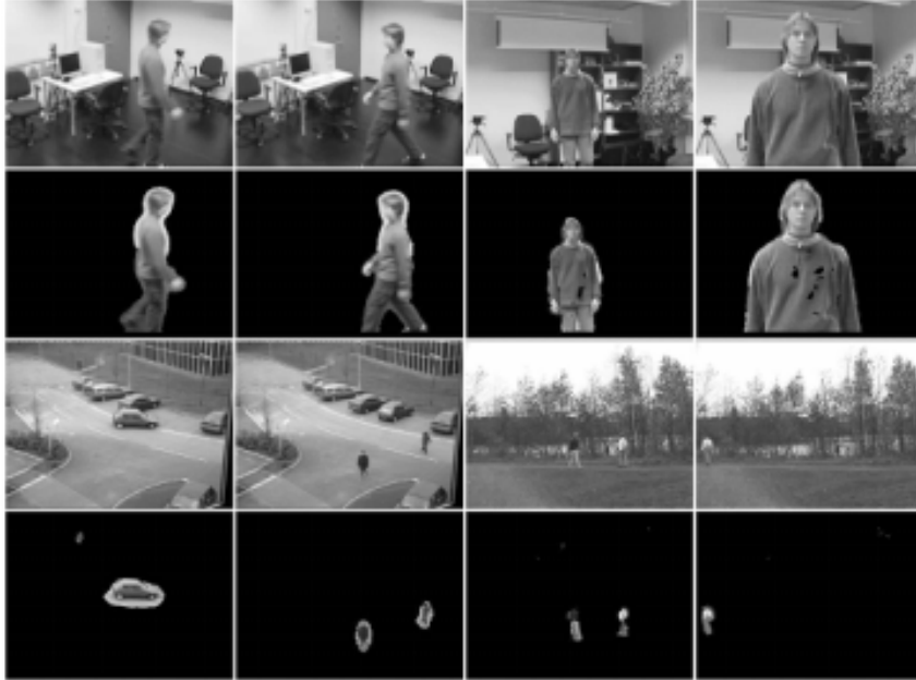
Fig. 4. The background subtraction results based on the method proposed by Heikkilä et al. [14]. The first and third rows are the test images. The second and fourth rows are the detection results. (Figures courtesy of Marko Heikkilä [14])
