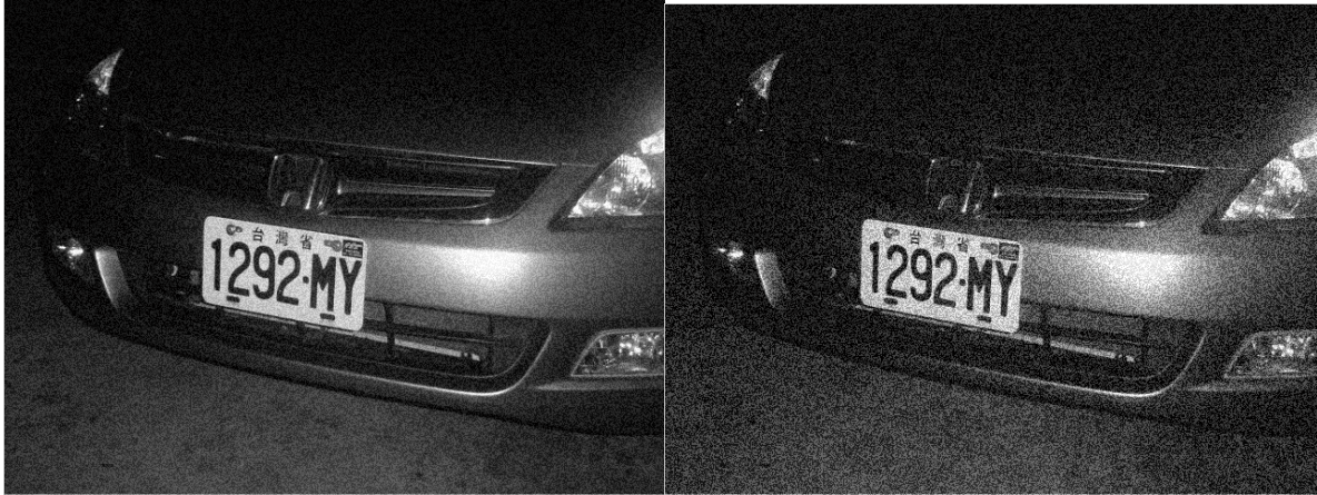
Fig. 6-3 Images used in noise analysis(left: 12.8%, right:25.6% quantization noise)
