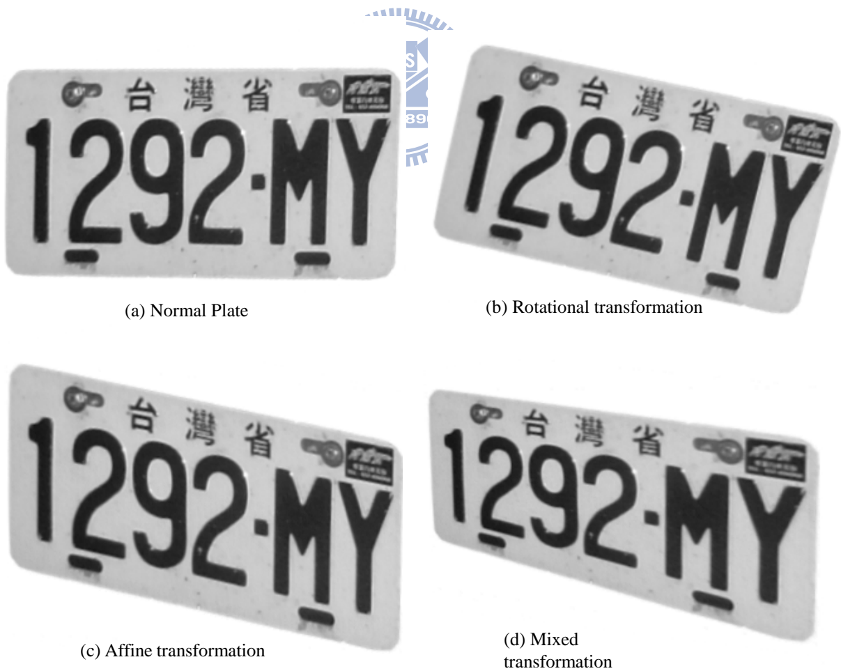
Fig. 4-1 Typical geometric transformations in LPR systems
