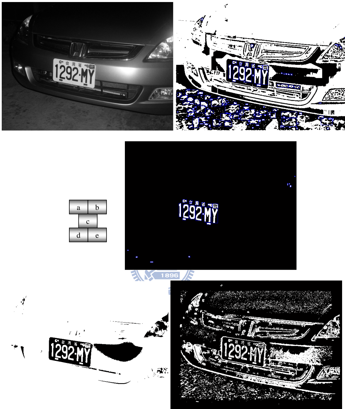
Fig. 6-1 (a) Source image#1. (b) Converted binary image; blue rectangles are isolated groups (c) Results after elimination, blue rectangles are character candidates. (d) Binarization result using Otsu's method. (e) Binarization result by LIG.
