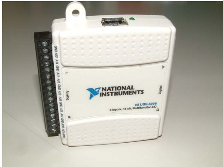
Figure 3-5 National Instrument USB-6009 A/D data acquisition device.
