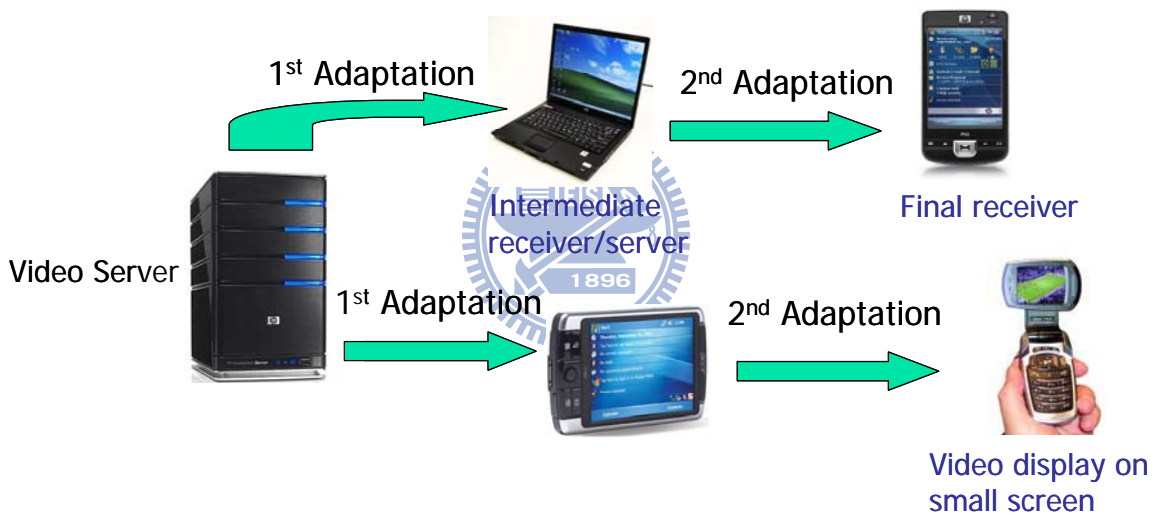
Figure 3-8: Two examples of multiple adaptation applications where the same video content is adapted several times down the distribution chains
