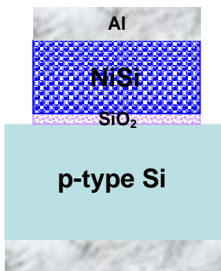
Fig. 6.9 Key process flow and schematics of the full nickel silicide MOS capacitor formation based on stack structure.
