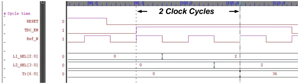
Fig. 3.9: Simulation of 2-level flash TDC.
