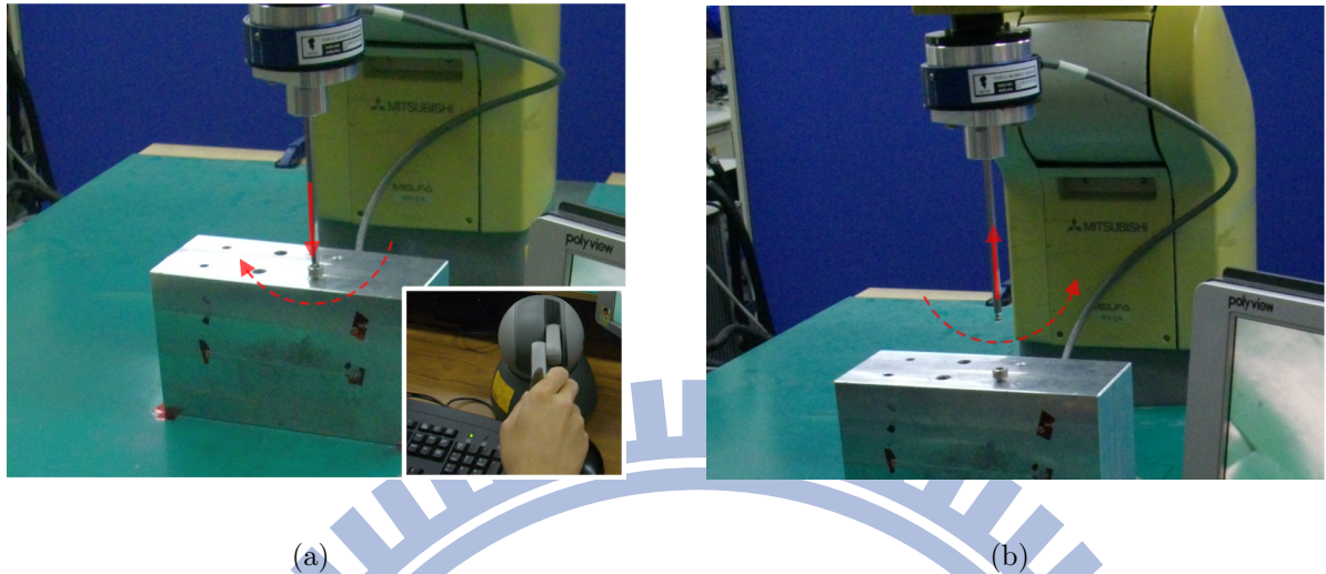
Fig. 3.12: Experimental setup for manipulating the hex key for screw fastening: (a) place the ball end of the hex key into the hex socket screw and turn it clockwise to fasten the screw and (b) release the hex key from the screw by turning it counter-clockwise.
