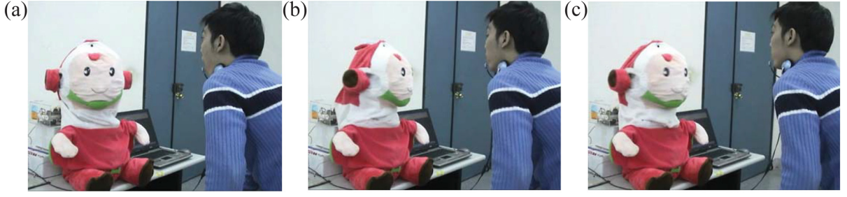
Fig. 4-16: Interactive response of the robot, when the user speaks in a surprised tone. (a) The robot shakes its head to the right. (b) The robot shakes its head to the left. (c) The robot puts its head back to the original position.
