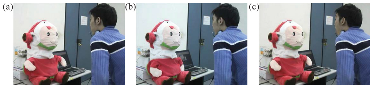
Fig. 4-15: Interactive response of the robot as the user says, “I am angry!” (a) The robot puts down its hands to portray fear. (b) The robot continues to put down its hands to the lowest position. (c) The robot raises its hands back to the original position.
