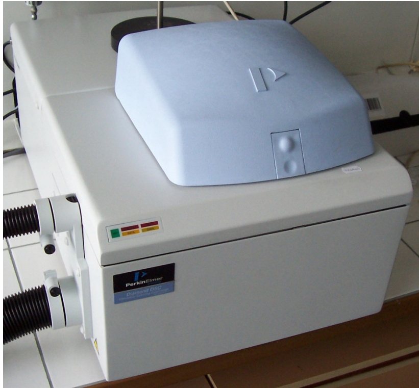
Figure 3.4 Differential scanning calorimeter (Diamond DSC, PerkinElmer Inc.) in the Department of Material Science and Engineering, NCTU.
