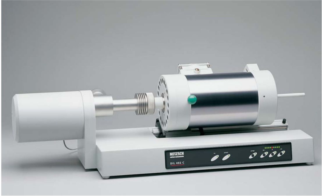
Figure 3.1 Dilatometer (DIL 402C, Netzsch) in the Center of EMO Materials and Nanotechnology, NTUT.
