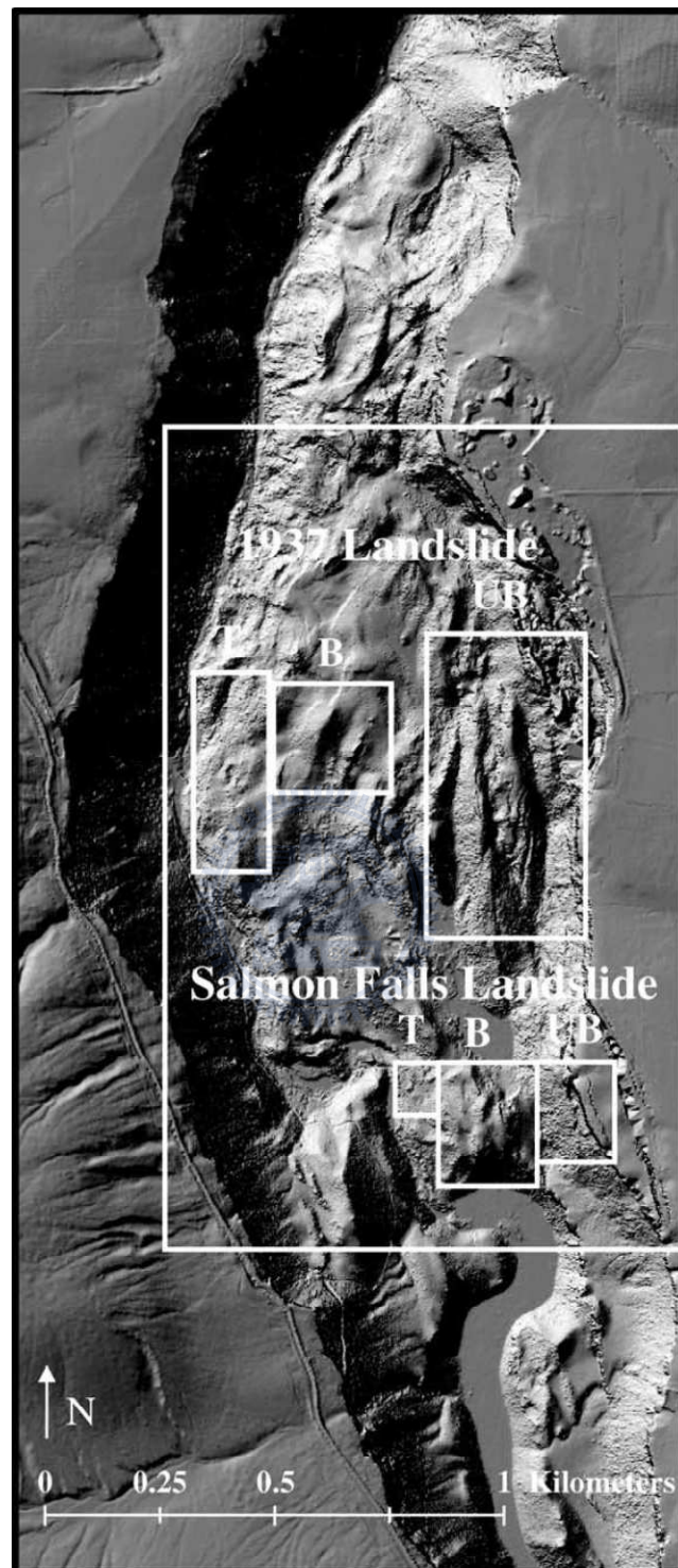
Figure 3.18 Shaded relief image of the Salmon Falls landslides for semivariogram and fractal analyses. UB=Upper block, B=Body, T=Toe.
