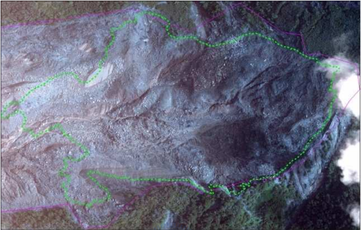
Figure 3.25 A close-up of the depletion area of Hsiaolin Slide. Remnants of unconsolidated materials still existed on the bare surface. The dash-line is the isoplethic line with -20 m. The area covers 48.68 hectares.
