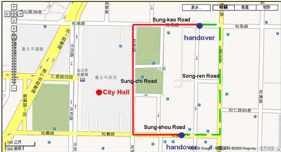
Figure 4.8 Moving Path for Mobility Tests (the solid path is covered by one base station, and the dashed path is covered by another base station)
