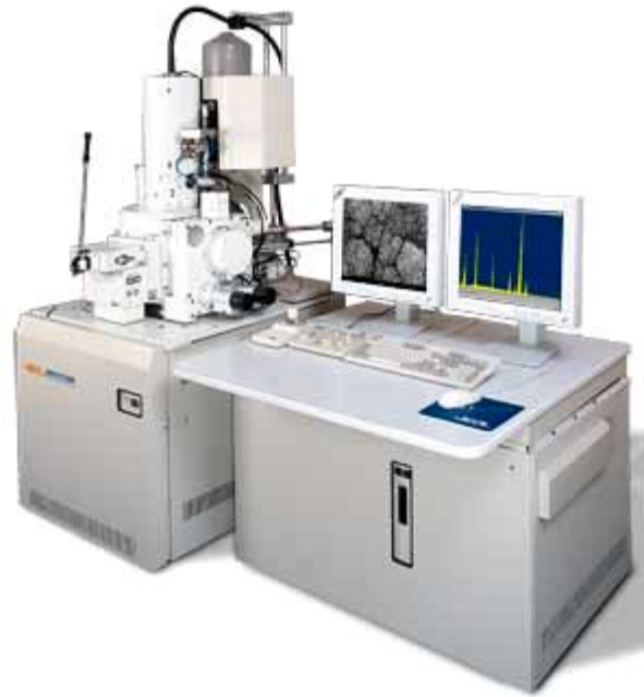
Figure. 3-5 systematically illustration of JSM-6700F HR-SEM
