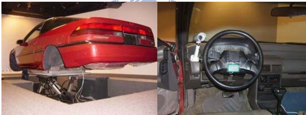
Fig. 2-1: Pictures showed the dynamic VR driving environment, in the Brain Research Center of National Chiao Tung University, Taiwan, and ROC. A real car in the 3D VR environment was showed in the left picture. The experimental setup around the steering wheel was showed in the right picture.
