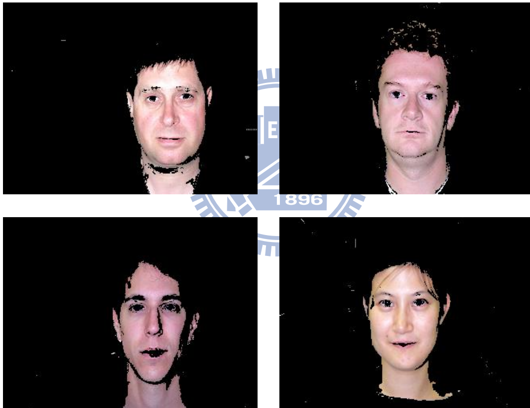
Figure 4.9: Results of skin color detection with 3 dimension input (Y, Cb, Cr).
