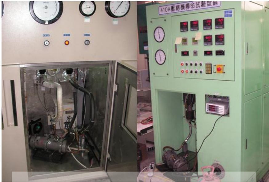
(a) Testing of semihermetic horizontal R410A STC prototype
