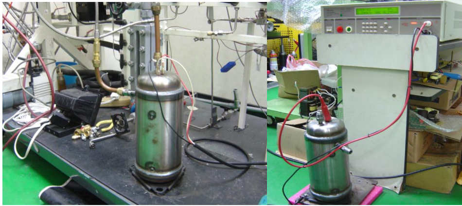
Fig. 5.18 Testing of R744 LPS hermetic STC for CO 2 heat pump water heater application
