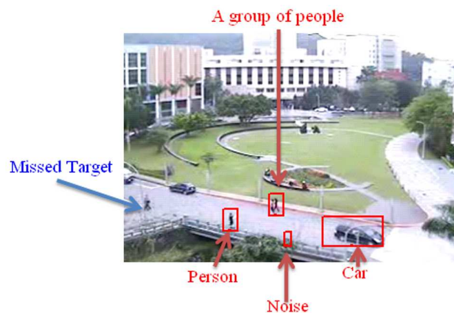
Figure 3.7: Detected targets (a single person, a group of people, a car, and noise)
