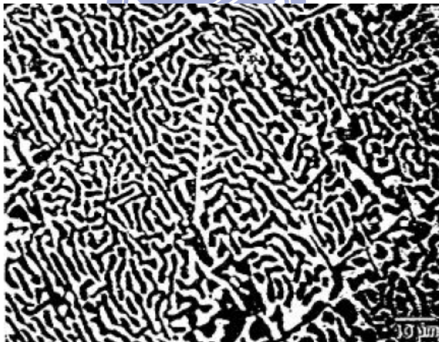
Figure 2.2 Microstructure of eutectic Bi-Sn alloy [3].
