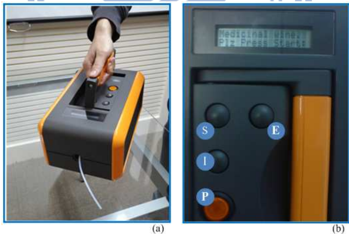
Fig. 5-25: Optical pictures of a portable E-Nose system: (a) the whole equipment, and (b) its control panel. (P = power On/Off, I = system initialization, S = training/testing mode selection, E = enter)
