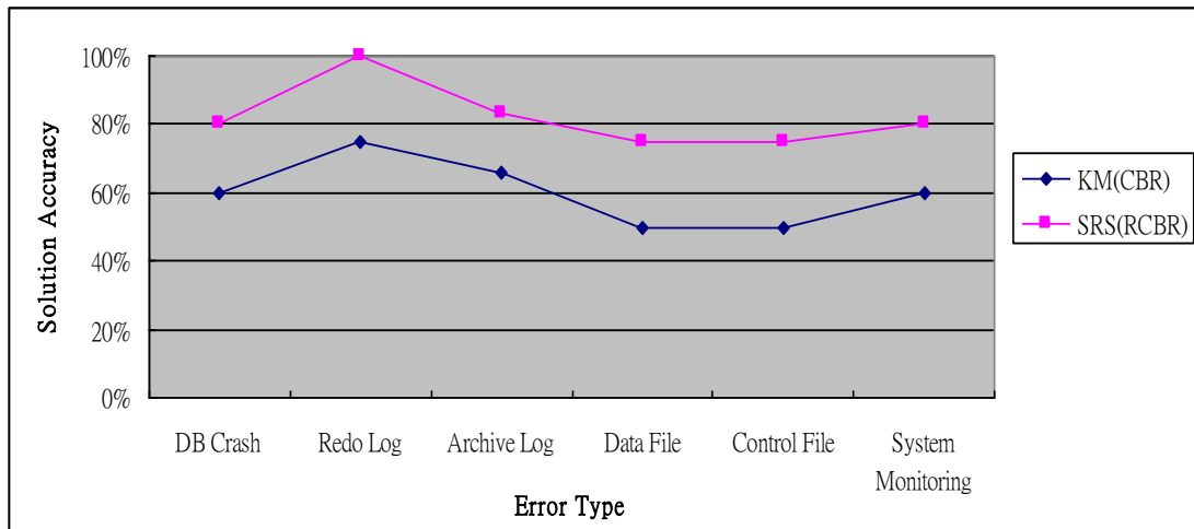
Figure 7.8 Accuracy evaluation between SRS system and KM center
