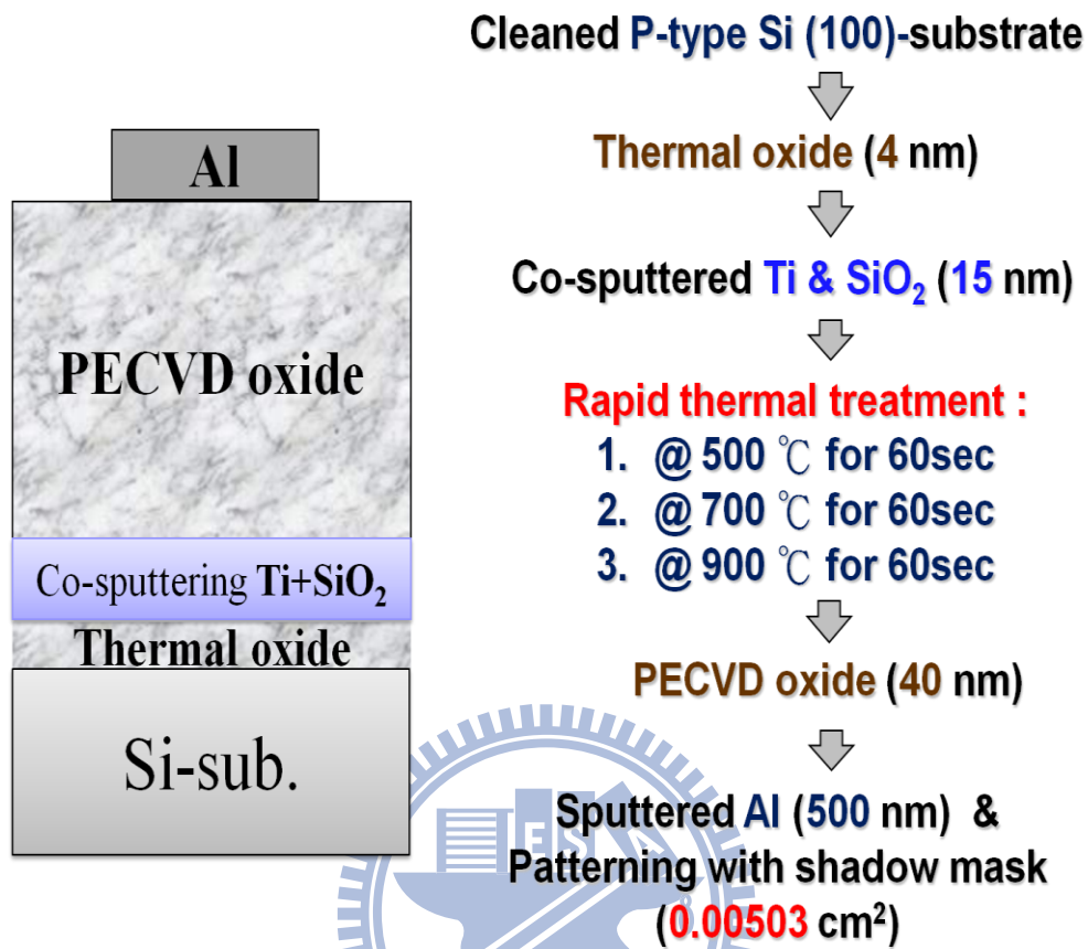
Fig. A-1 Illustration of the proposed titanium oxinitride nanocrystals device structure and process flows.
