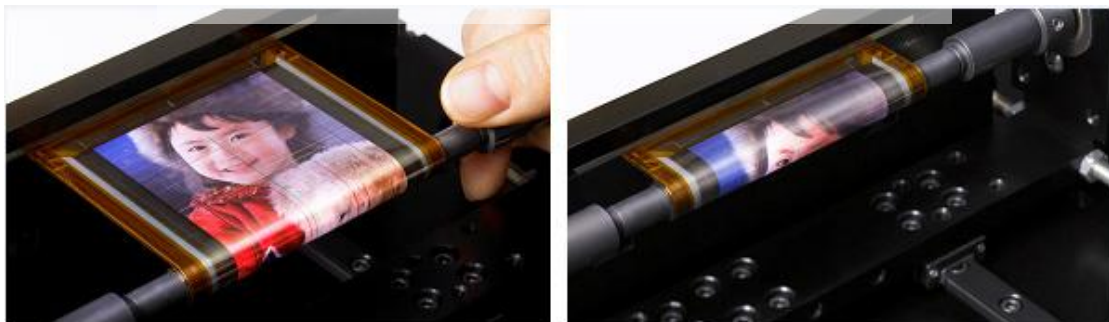
Figure 1-2 Photo of OTFT-driven OLED display wrapped around a cylinder with 4 mm radius. (Sony Corp.)
