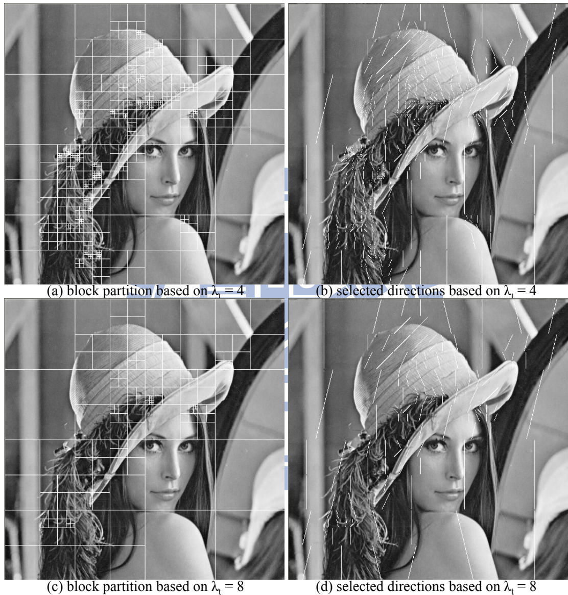
Fig. 2-13. Block partition and selected directions of test image Lena after rate-distortion optimized segmentation based on different Lagrangian multiplier \lambda_t .
