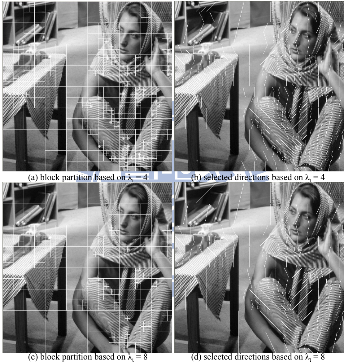
Fig. 2-12. Block partition and selected directions of test image Barbara after rate-distortion optimized segmentation based on different Lagrangian multiplier \lambda_t .
