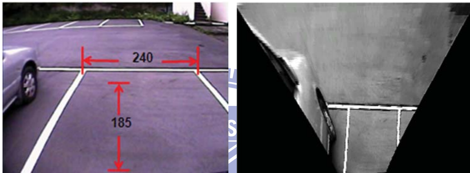
Figure 58: Scale measure between world coordinate and real length
