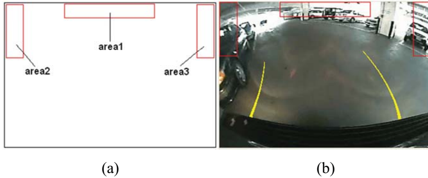
Figure 61: Allocation of motion detection areas.
