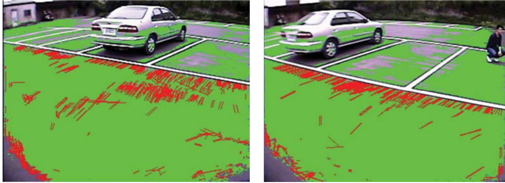
Figure 35: Results of feature point extraction. The upper image is result of road detection, and lower image is position of feature points.
