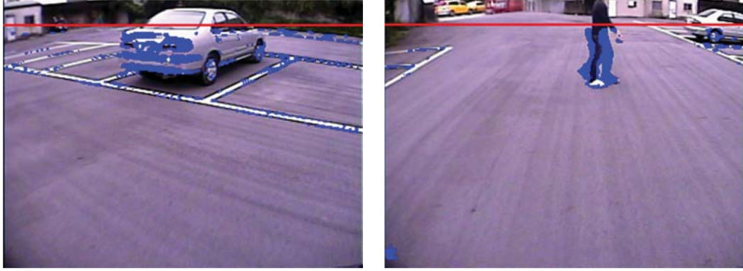
Figure 52: Results of image difference between current image and compensated image
