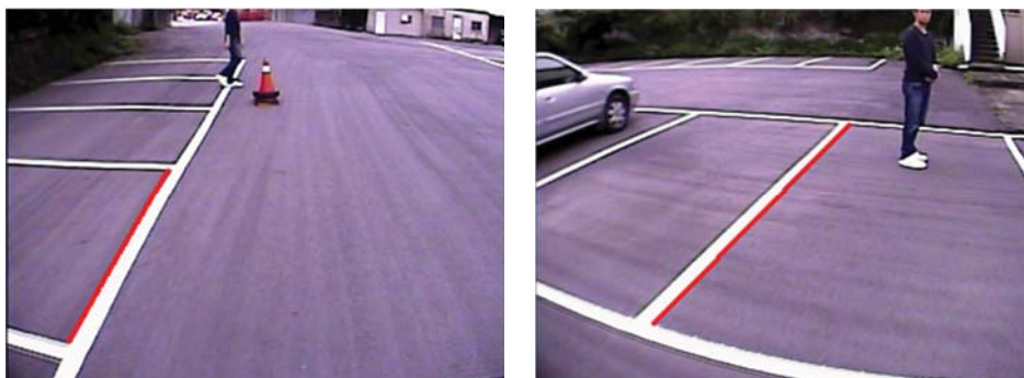
Figure 72: Lane marking for distance measurement
