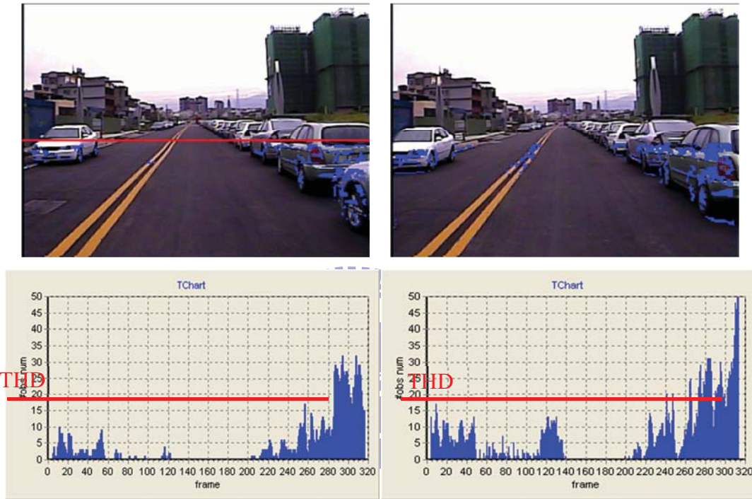
Figure 54: the obstacle candidate image and the corresponding vertical-orientated histogram
