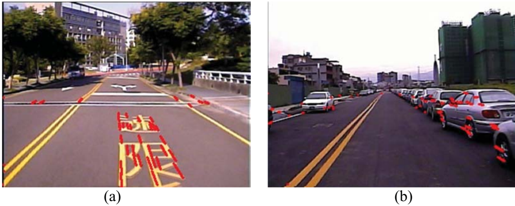
Figure 29: Results of corner detection and its corresponding optical flow
