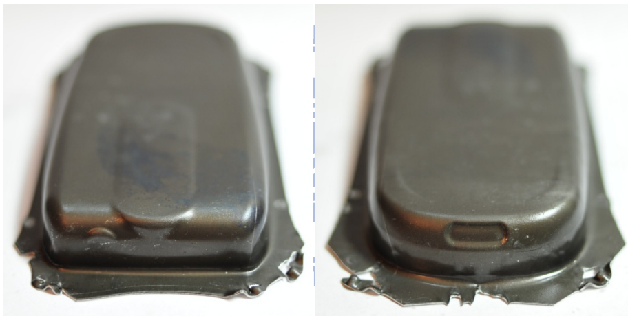
Figure 4.47 The Ti / Al clad metal sheet without failure (HF= 0.7 ton, chamfer width: 20mm)
