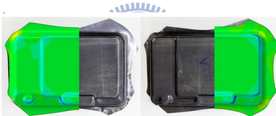
Figure 5.7 The deformation comparison of Ti/Al clad metal between simulation and experiment
