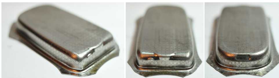
Figure 4.40 The deformation of SUS 304 with mesh (holding force: 2 ton, chamfer width: 20mm)
