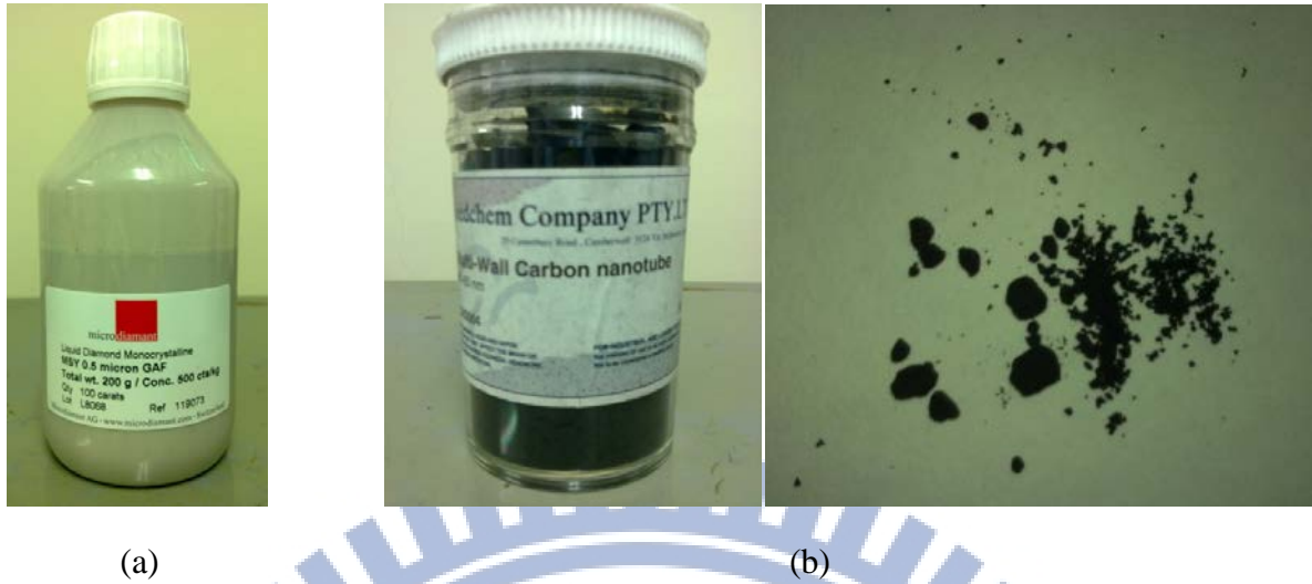
Figure 3.1 Nano particles for nanocomposite electroplating: (a) nano diamond particles in the preservation solution and (b) carbon nanotubes (CNTs) powder.
