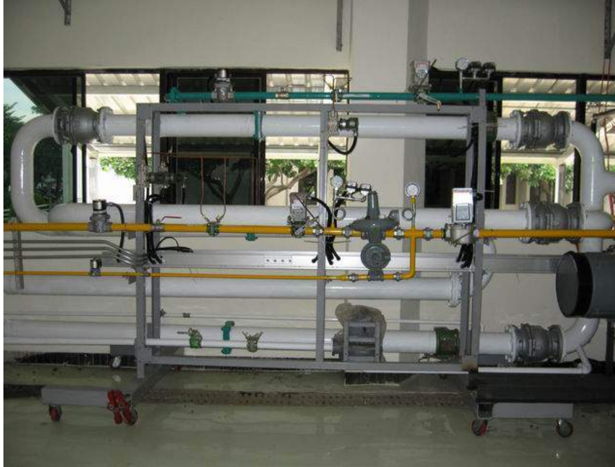
Figure 2.11 The Picture of pipeline control system (Pilot-Scale)
