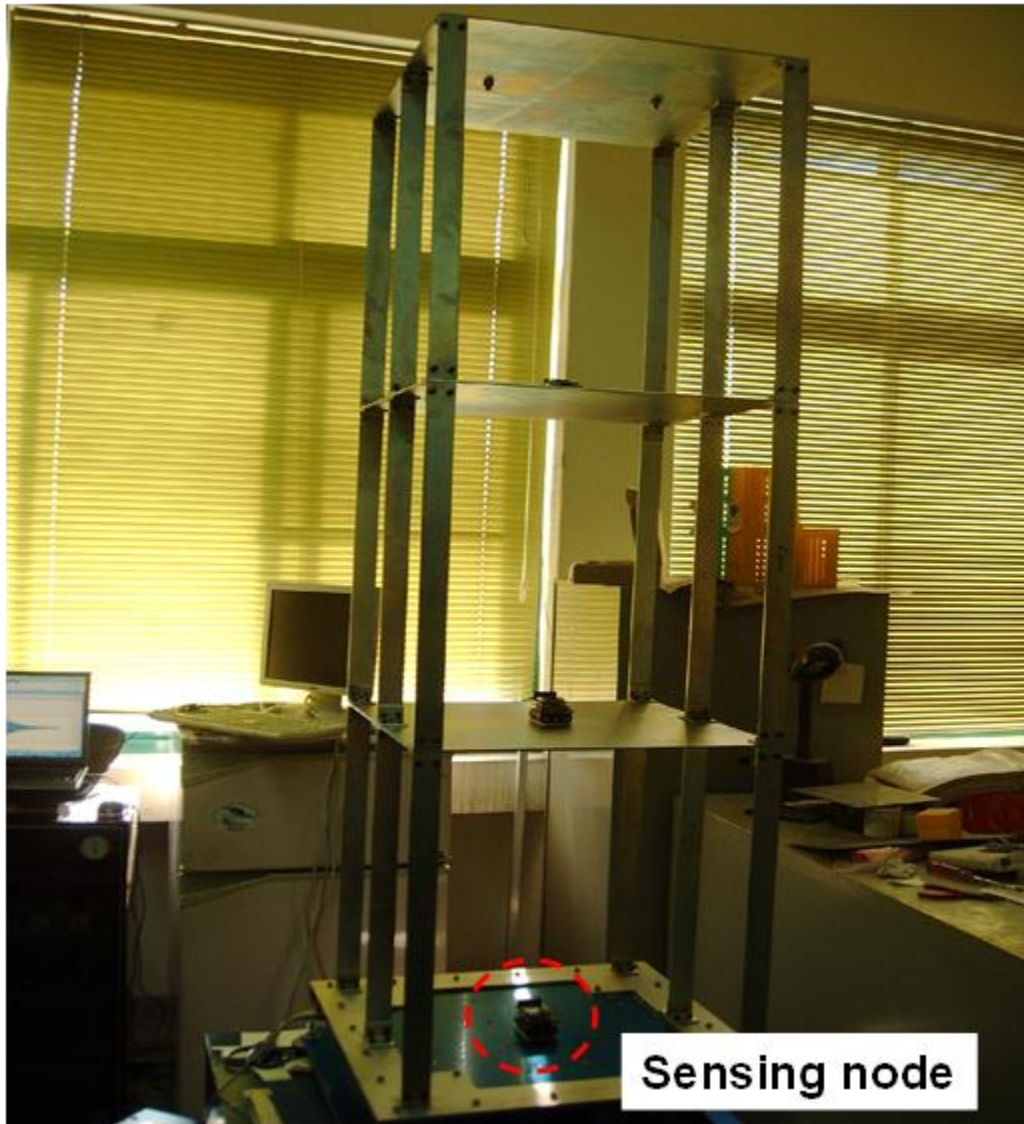
Figure 6.4 A 1/8-scaled three-storey steel frame model.
