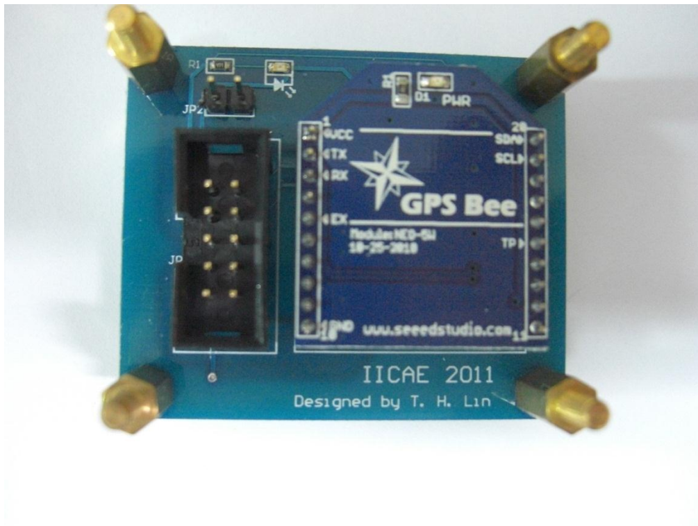
Figure 4.8 Photography of developed Multi-sensor board
